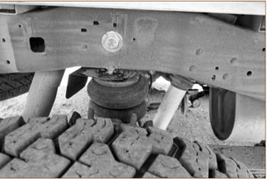
**Photo 2:** The Fremont County spray truck rides on an adjustable air bag and shock suspension that irons out spraying over the roughest terrain.
