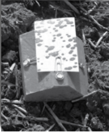
Multiple water sensitive papers (WSP) were used to collect spray droplets across the swath width for each treatment.
