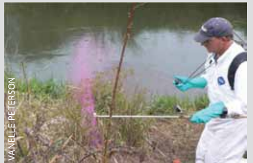
FIGURE 3: HERBICIDE APPLICATION at the Oregon flowing water research site. Total width of the application pattern was 15 feet, with 12 feet over soil/vegetation and 3 feet past the edge of stream bank (over vegetation in water and/or directly over water).
