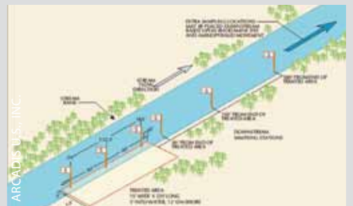
FIGURE 2: DIAGRAM of herbicide application and sampling in flowing water dissipation sites.
